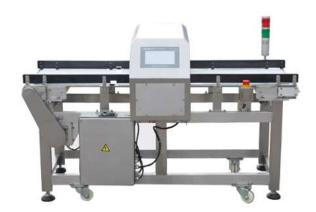
1. Product Features:Operating system adopts highly human-oriented and intelligent design and has the function of one-bottom self-learning. The machine can set and store product parameters automatically and precisely when the products to be detected passing metal detector according to set procedure, no need to adjust by human and is easy to operate.
